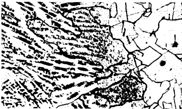
20% Cold Reduction and Annealed
