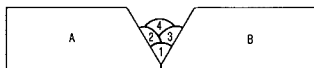
Figure 20. Multiple-pass dissimilar weld. Bead 1 is 15% A, 15% B, 70% filler metal. Bead 2 is 15% A, 15% B, 70% filler metal. Bead 3 is 15% A, 15% B, 70% filler metal. Bead 4 is 15% A, 15% B, 70% filler metal.
