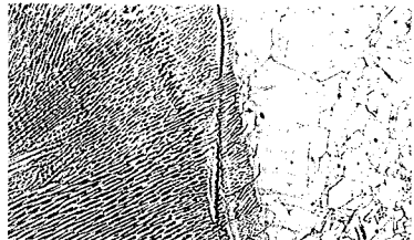
10% Cold Reduction and Annealed
