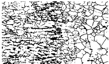
INCONEL Filler Metal 82 on INCONEL alloy 800
